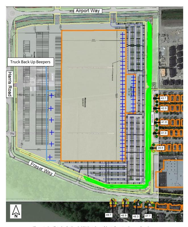
Figure 3 - Predicted noise levels (dBA) at the residents from truck reversing alarms
