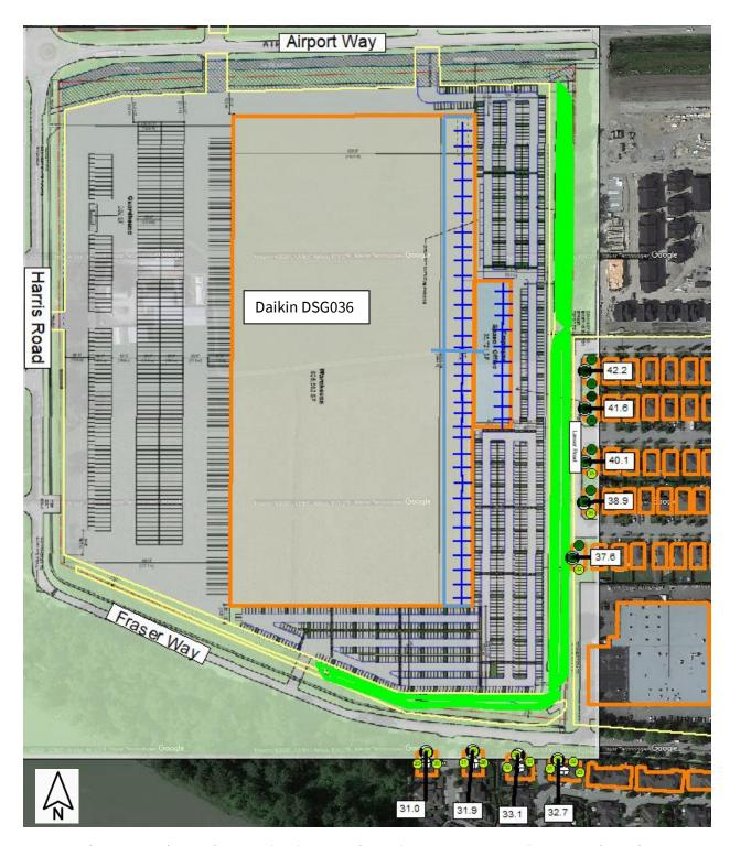
Figure 2 - Predicted noise levels (dBA) at the residents from the assumed rooftop mechanical units
