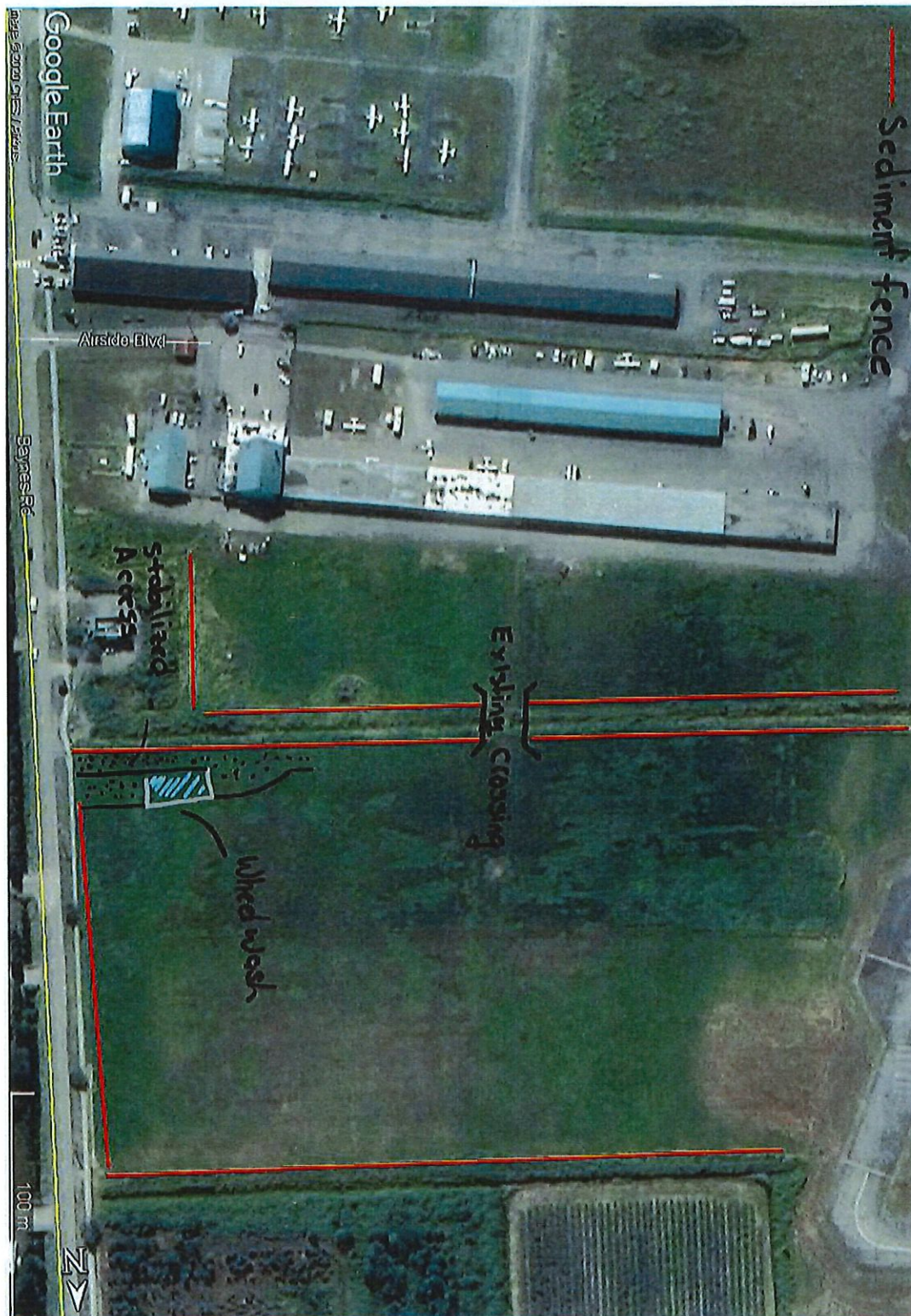
Figure 4. Proposed placement of ESC measures.
