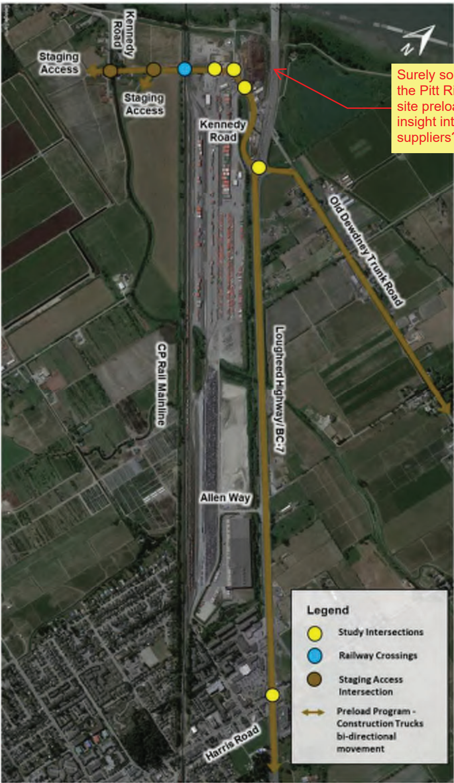
Figure 4-2: Truck Trip Distribution during the Site Preload Program
