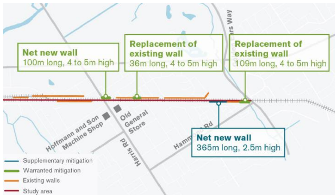
Figure 3 – Warranted + Supplementary Mitigation Walls (Port authority, 2021)
