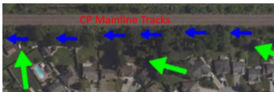
Figure 3 – Existing drainage paths of select properties adjacent to tracks, CP/Hatch, 2021 with City Edits
